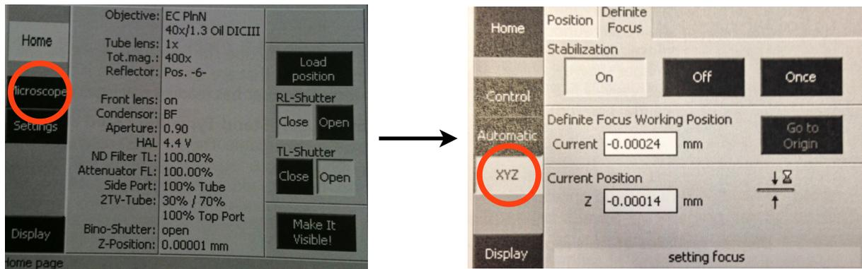
Definite focus allows different offsets to be used in time-lapse experiments using multi-positions. To enable this feature use **advanced features** in the **Image Capture** window. If using different offsets for multi-positions click "compute offsets".
