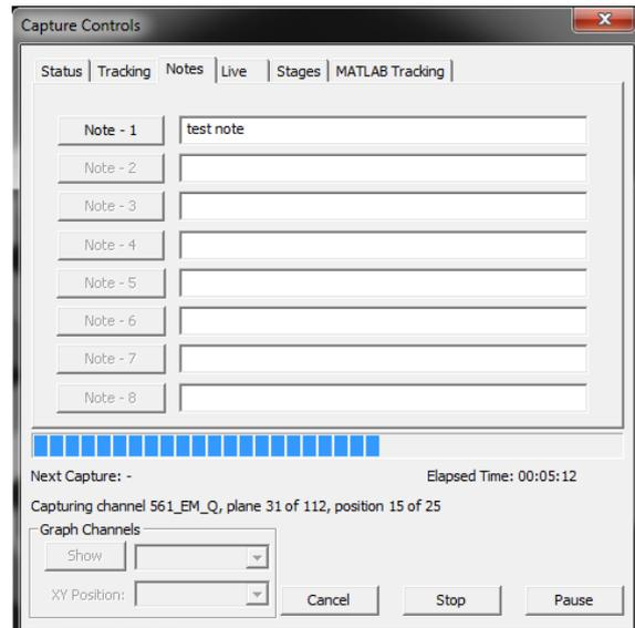
7. The **Status** tab of the **Capture Controls** window shows the progress of the multi-dimensional acquisition. The **Notes** tab can be used to mark events during the acquisition.
