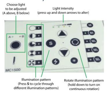
When using transmitted or incident light ensure you are using an empty filter turret position (positions 4 and 5)
