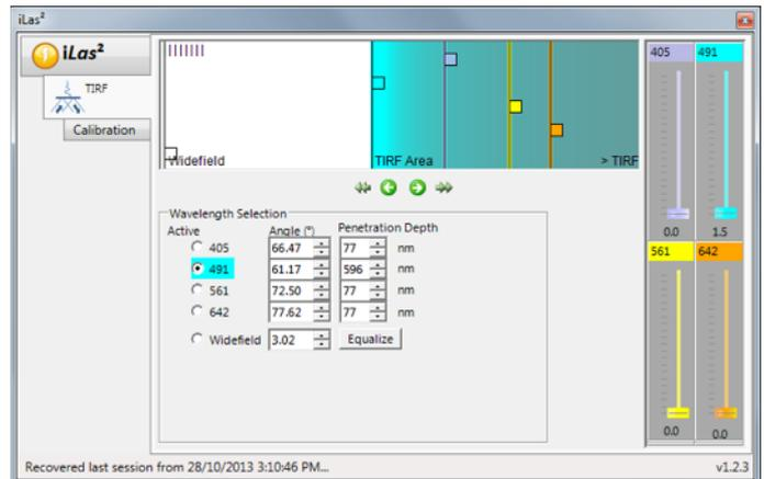
3. The currently active laser, the calculated angle and penetration depth are displayed in the **Wavelength Selection** panel. If multiple laser lines are defined in the Illumination configuration these are controlled using the **Widefield** slider (in white).
