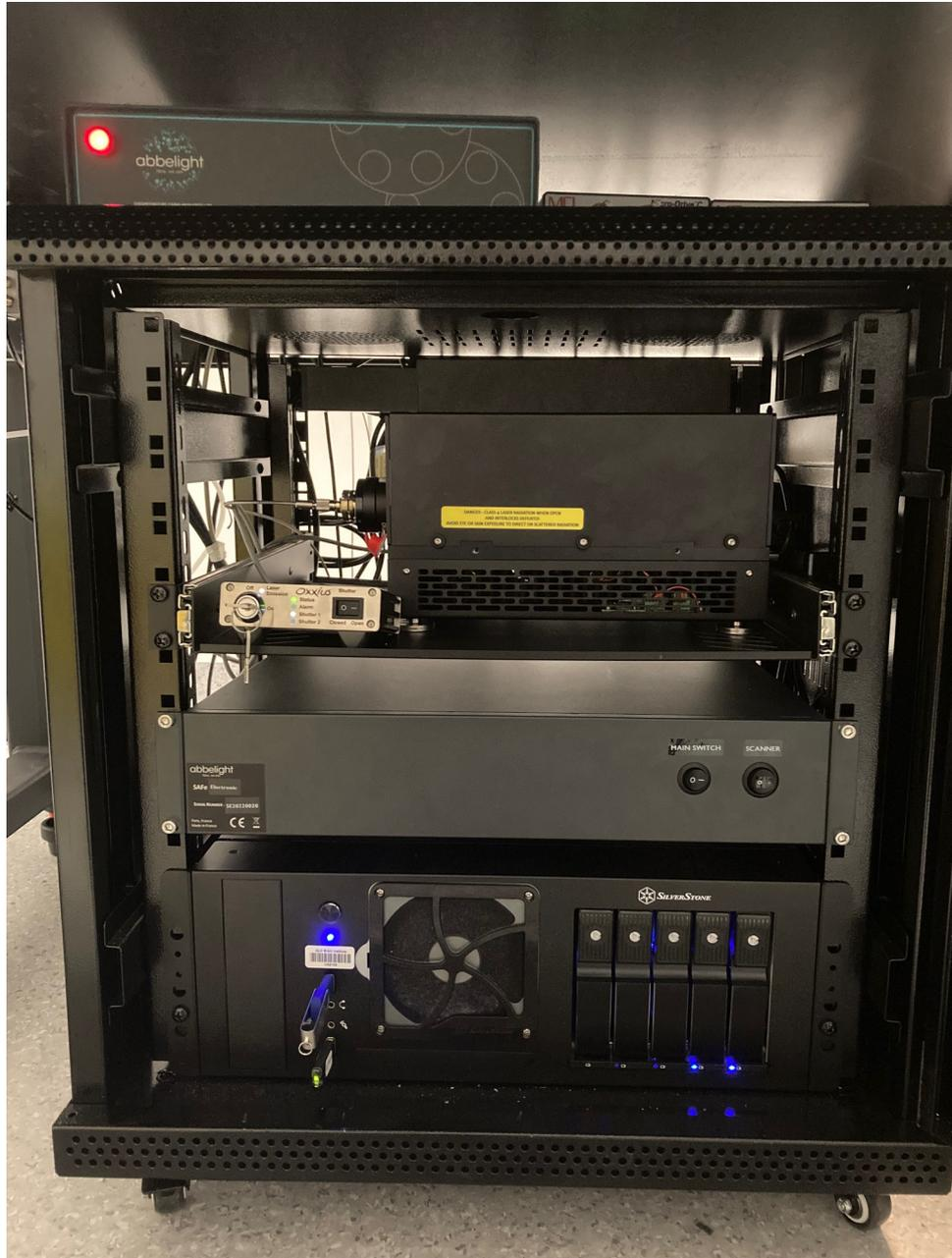
Figure 4: Abbelight tower showing (top to bottom): Abbelight module, Oxxius laser controller, SAFe Electronic module, and acquisition PC.
