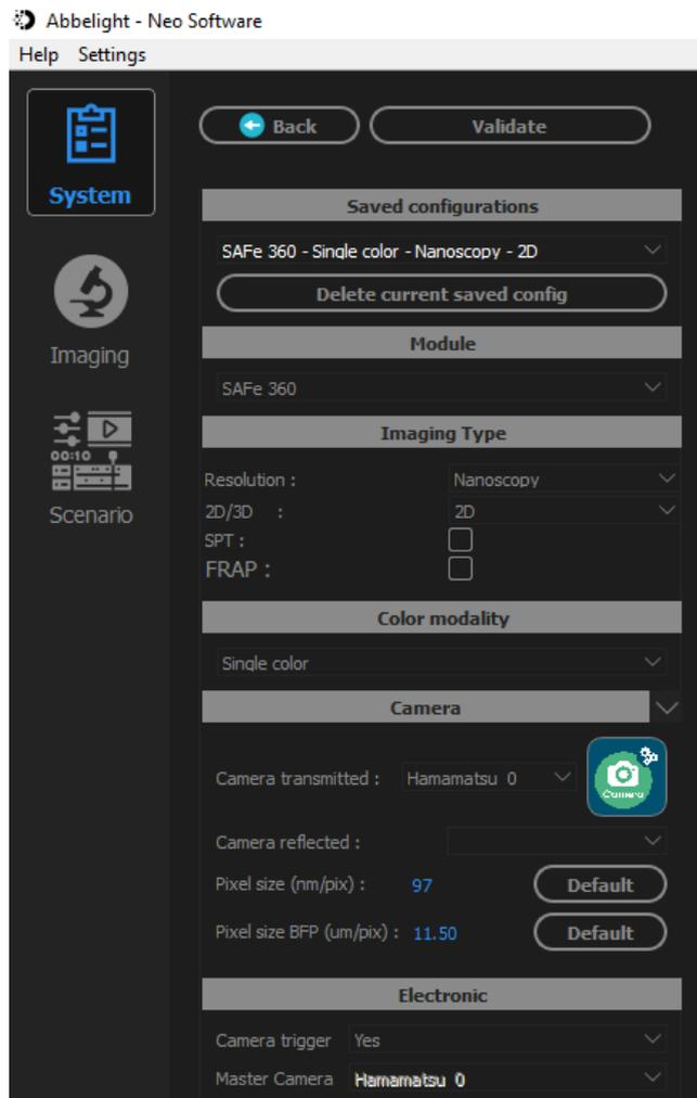
Figure 23: The hardware configuration window for single-channel acquisition of far red signal. The master camera must be set to “Hamamatsu 0.”
