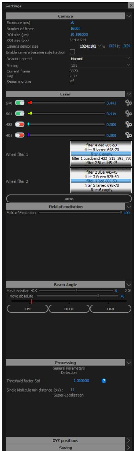
Figure 12: Setting the acquisition parameters.
