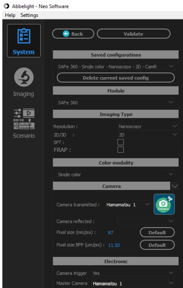
Figure 24: The hardware configuration window for single-channel acquisition of red, green, or blue signal. The master camera must be set to “Hamamatsu 1.”
